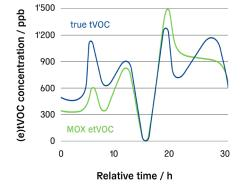
The plot above shows a typical field situation for VOCs. Due to its nature, the etVOC output of a typical MOX sensor deviates significantly from the true tVOC concentration. Some events may even not be detected by the MOX sensor if it is not sensitive enough to this particular VOC.
