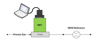
Figure 4 Recommended configuration for re-calibration of Mass Flow Controllers
