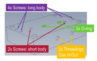
Figure 3 Suggested manifold design for SFC53xx / SFM53xx
