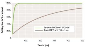
Figure 6: Settling time of the SFC5400 vs. typical thermal mass flow controller.
