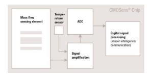
Figure 1: CMOSens® flow sensor diagram.
