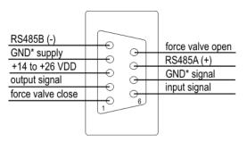
Figure 10: Analog interface versions (0-5VDC, 0-10VDC, 4-20mA) with auxiliary RS485 interface for extended functionality. RS485 interface is for service purposes only, e.g. it is not possible to set the set point using RS485. These versions have order codes "Q", "R", and "S" respectively (see Sec.0). Note that the pin layout of this version is not compatible to our analog only devices shown in Figure 9. \*GND pins are interconnected on the PCB of the device.
