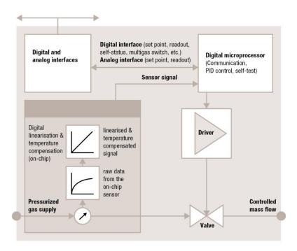
Figure 2: Block diagram CMOSens® SFC5400 mass flow controller.
