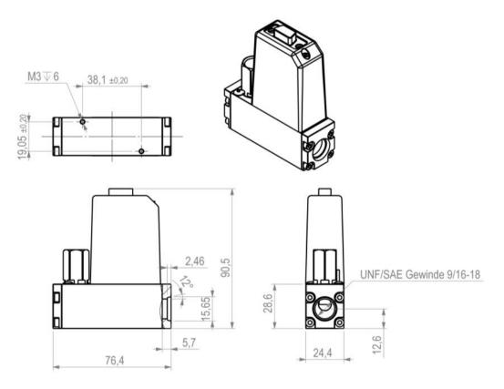
Figure 11: Physical dimensions and mounting information for the fitting versions. Specific dimensions for different types of fittings are shown in the next figure. All units are in [mm].
