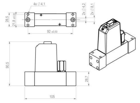
Figure 13: Physical dimensions and mounting information for the downmount version. All units are in [mm]. Recommended O-ring: NORMATEC O-ring FKM NT 80.7/75 OR 2019 inner Ø 4,76 x 1,78 mm
