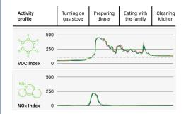
The figure at the top demonstrates a possible example implementation of the  $NO_x$  Index in an air purifier. At the bottom, one can see a typical activity profile in a kitchen for which the simultaneous monitoring of VOC and  $NO_x$  Indices helps distinguishing different types of events.
