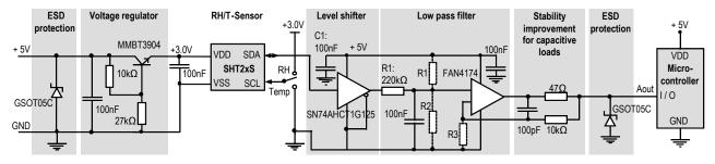
Important note: Capacitor C1 (100 nF) and resistor R1 (220 k $\Omega$ ) should be placed <u>as close as possible</u> to the driver (SN74AHCT1G125) to minimize noise on analog output signal Aout.
