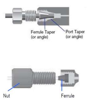
Note that nuts on the flat bottom ports should only be tightened finger-tight if not specified otherwise in the sensor's datasheet.
