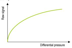
After the process of linearization, the sensor output is always a 16bit integer value, scaled with the sensor's scale factor of 60Pa-1. However, this 16 bit number is based on the internal digital resolution, which can be adjusted by the customer.
