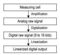
A higher resolution of the signal relates to a longer integration time, which delivers a smoother and more precise differential pressure value. A lower resolution relates to a short integration time, delivering measurement results with faster response times.
