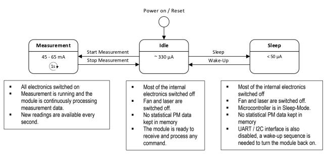
Figure 1: The different operating modes of the SPS30 PM sensor.
