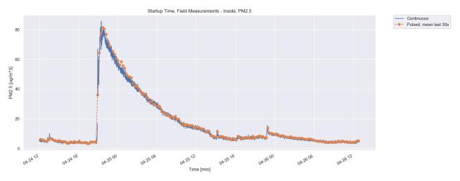
Figure 6: A typical indoor cooking event with fast increase and a slow decrease can be perfectly measured with the proposed implementation example. Blue curve: continuous measurement. Orange curve: 60 seconds measurement time represented by one data point as an average of the last 30 seconds, 15 minutes sleep time.
