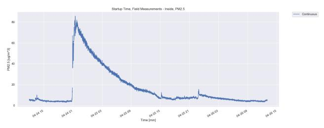
Figure 4: A typical indoor cooking event with fast increase and a slow decrease, measured in continuous measurement mode.
