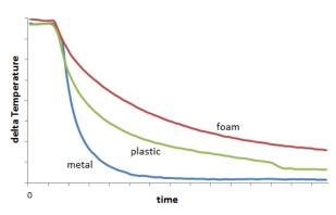
Figure 2 Exemplary data showing several sensors approaching reference value. Different materials have been used to couple the sensors to the reference sensor. Metal offers the best thermal coupling, resulting in the fastest settling times. Coupling sensors through e.g. plastic or foam requires significantly longer settling times and may lead to less accurate measurements.
