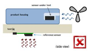
Figure 11 Bad example with reference sensor located far from the sensor under test. Reference sensor is exposed to hot air, while the sensor under test is cooled by a ventilator and/or air conditioning, creating a thermal imbalance. Neither sensor is shielded from turbulences.
