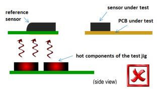
Figure 6 Bad example of PCB test jig. Sensor under test and reference sensor are not sufficiently close together and have to rely on the thermal coupling through air alone. Additionally, there are heat sources below the sensors creating a thermal imbalance.
