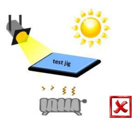
Figure 14 Bad example of a test jig that is exposed to different heat sources – direct sunlight, a strong spotlight and a heating system.
