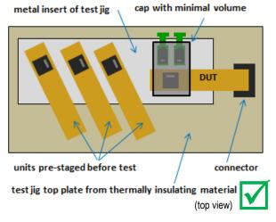
Figure 7 Good example of test jig top plate from thermally insulating material (e.g. plastic), preventing the operator to easily touch the metal insert of the test jig. The metal insert is large enough to provide space for pre-staging several units before test, allowing the units to adjust to the temperature of the jig.
