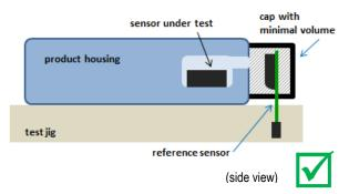
Figure 10 Good example of reference sensor mounted inside a cap, covering the sensor opening of the product housing. The volume inside the cap is minimized, at the same time protecting the sensors from turbulences in the environment.
