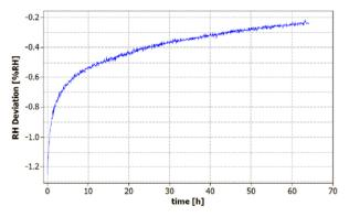
Figure 17 Mean deviation from initial calibration when sensor is exposed to ambient conditions of 25°C and 50 %RH directly after reflow soldering process (representative plot)
