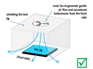
Figure 15 Shielding the test jig to the left/right/back/top reduce turbulences at the test jig. Access for operation is from the front side only. A small fan in the top cover ensures a gentle air flow towards the operator, further reducing the effect of turbulence near the jig.
