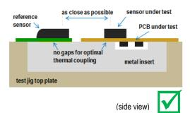
Figure 3 Good example of PCB test jig with a metal insert, ensuring good thermal coupling between the reference sensor and the sensor under test as well as a minimum distance between them.
